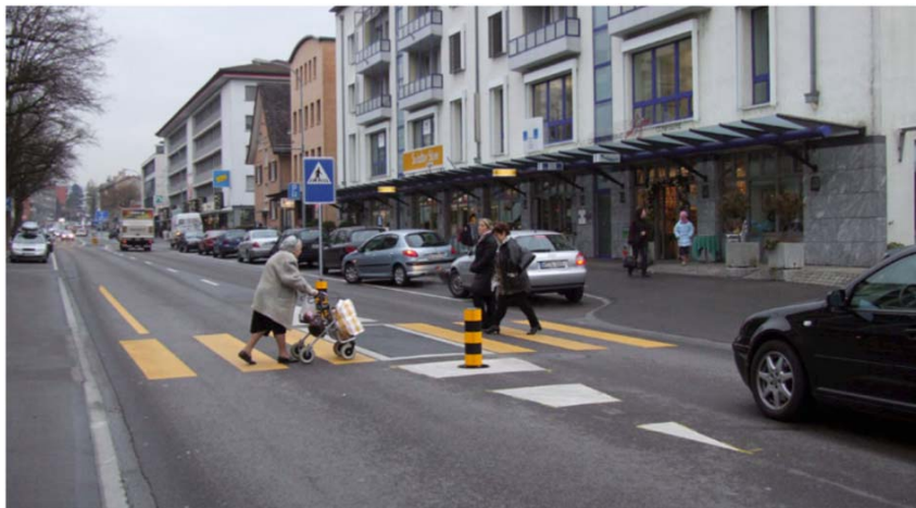
Figure 25 Ilot central marqué, Wettingen
